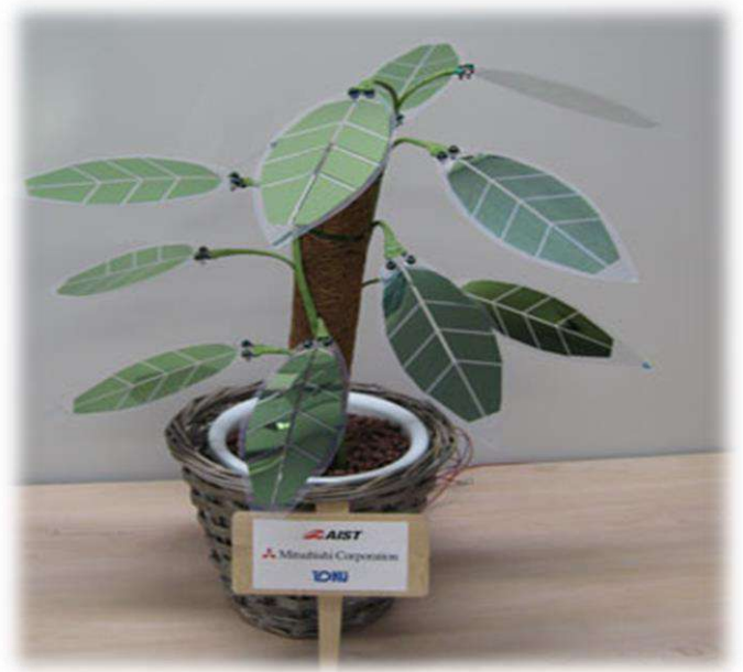
Figure 3. Leaf type Photo Voltaic Module
