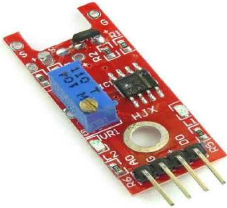
Figure 5 Hall Sensor Module
