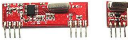
Figure 1 Transmitter – Receiver pair
