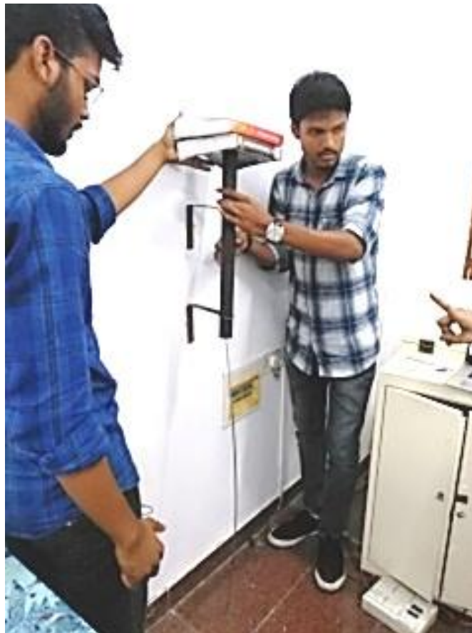
Students, testing their column under 5 kg load
