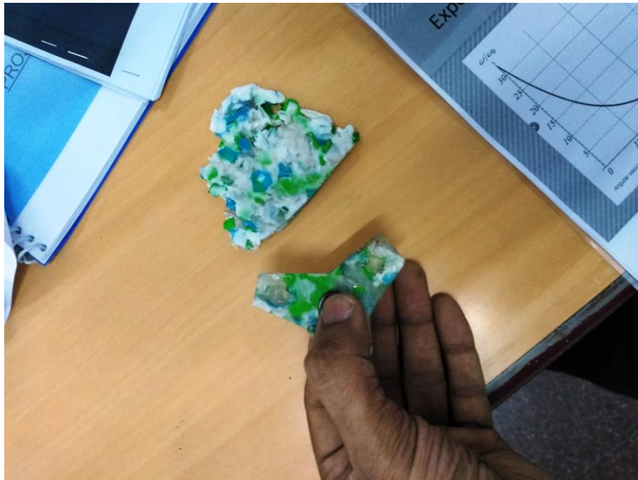
Use of plastic waste from used bottles, bags etc. to create fidget spinner body, by a Mechanical group of students
