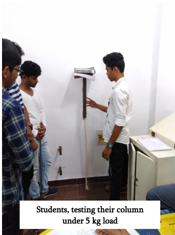
Students, testing their column under 5 kg load
