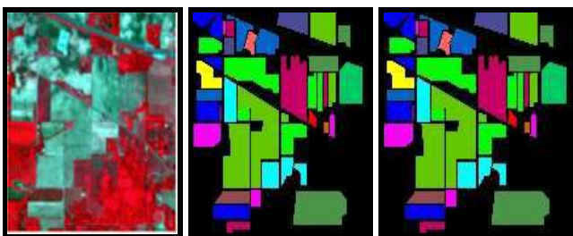
Fig. 4.1: The classification map for Indian Pines, (a) False color image (b) Ground truth (c) Predicted classification maps for proposed CNN model.
