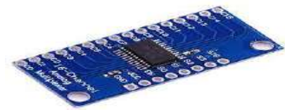
Figure 2 16-CHANNEL ANALOG MULTIPLEXER
