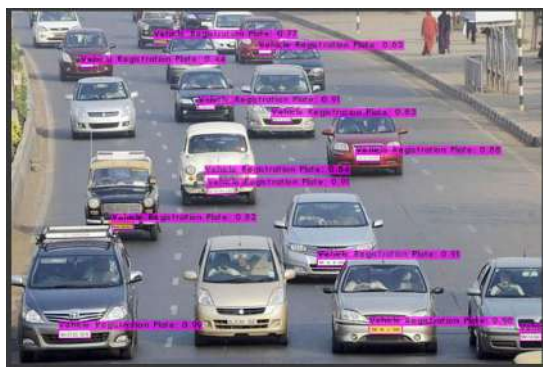
Fig. 5 Result showing the labelling of Number Plates for vehicles after training and detection using YOLOv4 technique over Open Image Dataset.
