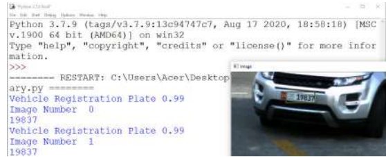
Fig. 6 Result showing accurate detection and recognition of the number plate from a video.
