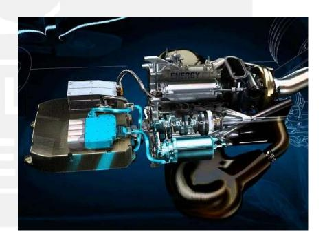
MGU-H captures the thermal energy generated from the exhaust gases from the engine, this thermal energy is also used to generate electric energy which is stored in the battery. Current regulations allow the electricity generated in MGU-H to be directly fed in MGU-K. Modern F1 cars heavily rely on the power generated by these electric units. MGU-H solves the problem of turbo lag by using a motor to power the compressor.
