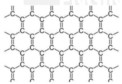
Graphene is the thinnest compound known to man at one atom thick, the lightest material known (with 1 square meter weighing around 0.77 milligrams), one of the strongest compound
