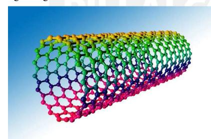
These nanotubes can be either single walled (SWCNT) or Multi-walled (MWCNT) with multiple rolled sheets linked in a concentric manner. With increased wear resistance, breaking strength, its antistatic properties along with its weight reduction capabilities, these are being planned to be used in future Aircrafts and Space shuttle missions, making it a trending material for
