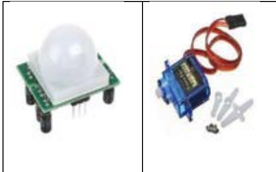
Fig.4: PIR sensor and Servomotor
