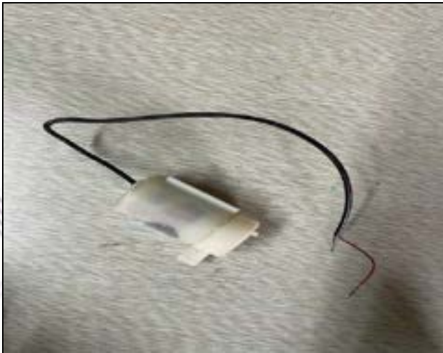
Figure 2: DC Motor ESC-208 DC3-6V(SUBMERSIBLE)
