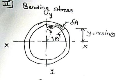
The moment of Inertia of an annular fillet weld is obtained by integrating above eqn.
